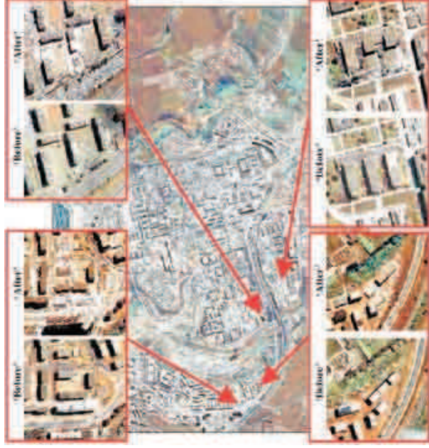
Figure 4.2.11: Example of earthquake damage assessment in Boumerdes, Algeria (Adams, 2004)
