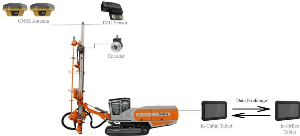
Figure 1-MG Installation Structure
