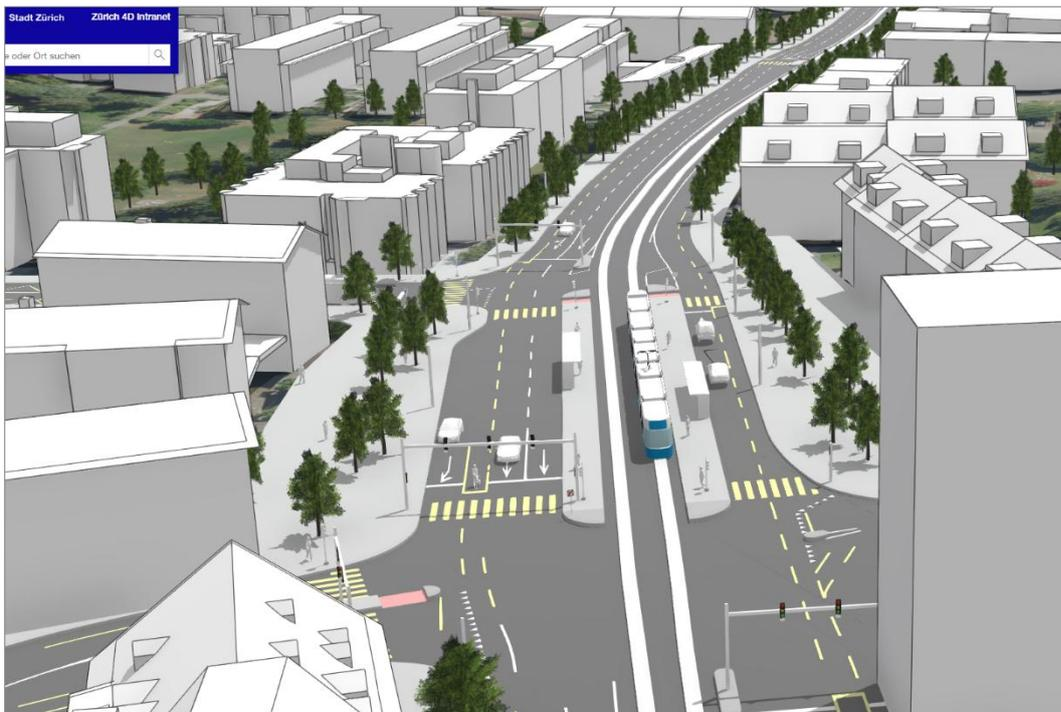
Figure 2 Project data for new tramline and street realignment, fusion of BIM data and existing 3D city model
