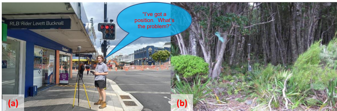
Figure 1: Examples of challenging satellite positioning environments: (a) in the vicinity of buildings including an overhanging veranda (staged), and (b) thick vegetation that interferes with the transmission of the GNSS signal.
