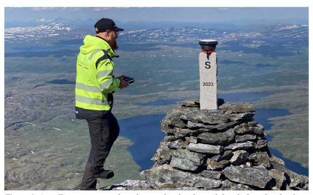
**Figure 6:** A small stone cairn as a boundary marker that do not define the boundary has been erected on the highest point along the boundary (1752 metres above mean sea level), here surveyed with network RTK by Swedish field engineer Karl Tirén.
