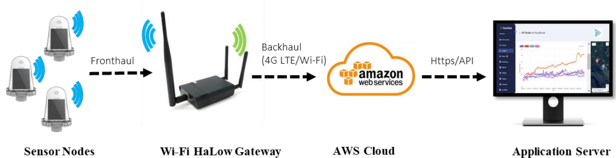
Figure 3 Diagram of data Wi-Fi Halow communication network.
