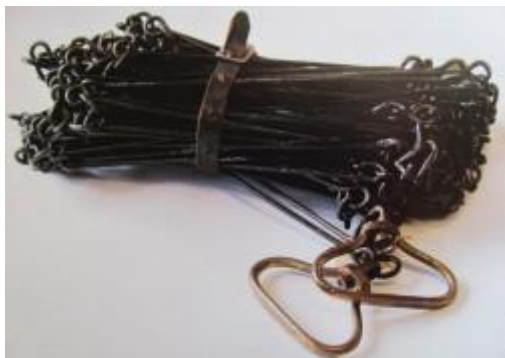
Picture 6. measuring chain
