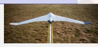
Parachute / Belly (skid) landing Carbon/Kevlar 60 km/h -25C between +45C L1&L2 PPK
