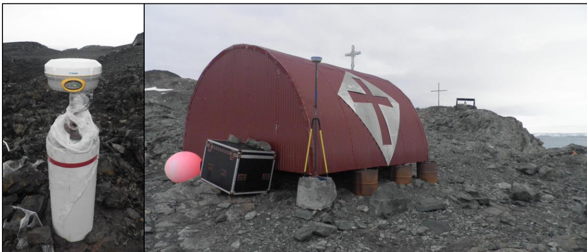
Figure 5 (a, b). a - Base receiver set up on the permanent GNSS marker KOH2; b – Rover receiver measuring the chapel's roof corners for TLS data georeferencing.
