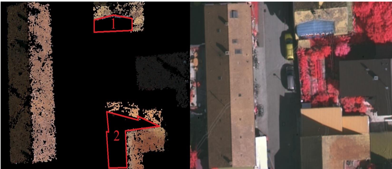
Fig. 4 The blanks on the roofs (1. The flat plane, 2. The falling over shadow of dense)
