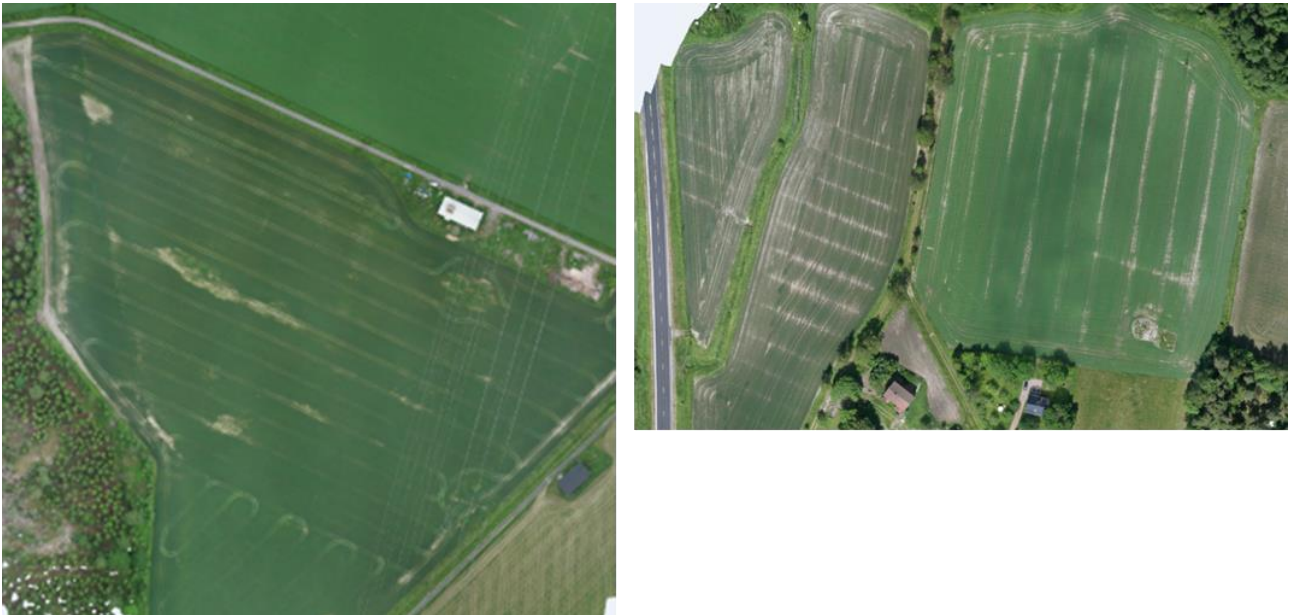
Figure 3. Parts of orthomosaics where the farmer can identify areas of ice encasements (left) and old sub-surface drainages (right)
