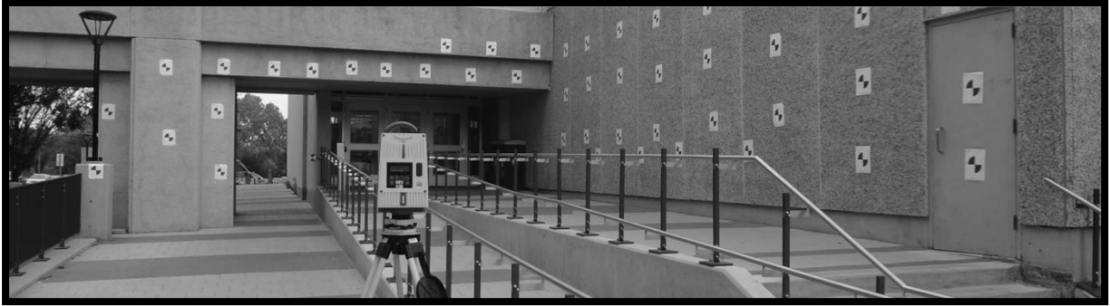
Figure 3.2: Point-based self-calibration set up showing Leica black-and-white targets placed on walls at the University of Calgary
