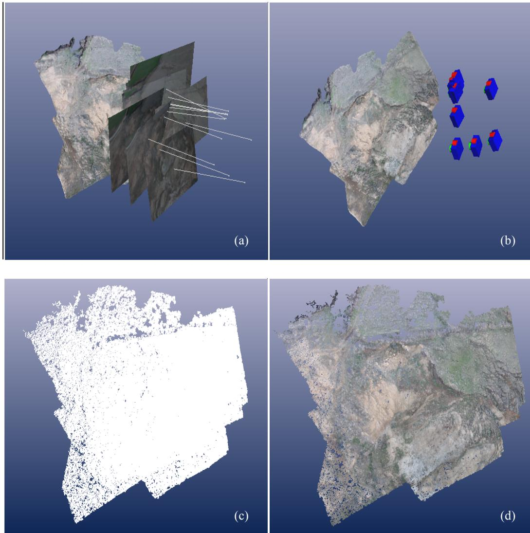
**Fig. 7:** (a): Image planes from UAV photos. (b): Image frustum plane. (c): Point cloud with single color. (d): Point cloud with exact color from photo.
