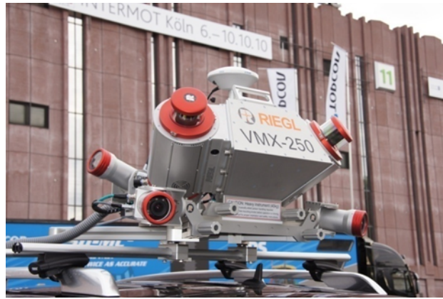
Figure 4. A Photo of Mobile Measurement System (MMS)
