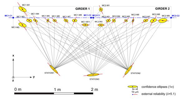
Figure 6. Microtriangulation Network measured with QDaedalus with the confidence ellipses and the vector of external reliability. The datum was fixed by minimizing the trace of the coordinates of all points on the modules.
