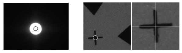
Figure 3. (Left) Example of a lamp measured by QDaedalus with center of mass. (Right) Example of a point measured by QDaedalus with template least square matching algorithm.
