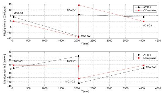
Figure 7. Misalignments in X and Z measured with the AT401 and QDaedalus .
