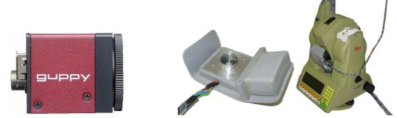
Figure 2. (Left) Guppy CCD camera as available on the market. (Right) Transformed CCD camera. The left picture shows the CCD sensor and the mechanical interface for Leica instruments. The right picture shows the camera mounted at the telescope of a TCA 1800. This adapted flat layout allows to measure even in zenith direction
