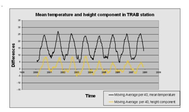
Figure 3. TRAB station's height component and temperature
