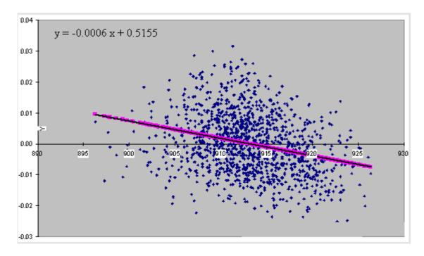
Figure 6. First part of ANKR Station regression line of height components with average pressure
