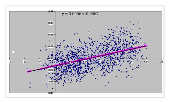
Figure 5. First part of ANKR Station regression line of height components with average temperature
