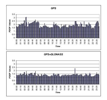
Figure 1. GPS and GPS/GLONASS PDOP values
