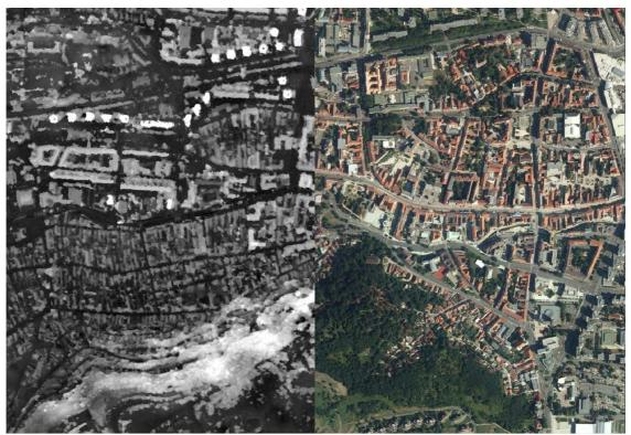
Fig. 3.: DSM and HUNDEM-5 differences (left) and digital orthophoto (right, Miskolc, Hungary)
