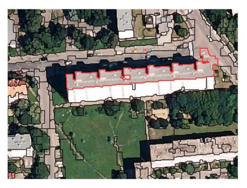
Fig. 7.: False classification of building based on density
