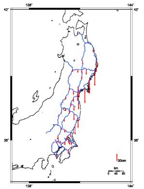
Fig. 6 Amount of displacement between revised Survey Results and the Geodetic Coordinates 2000 (vertical)
