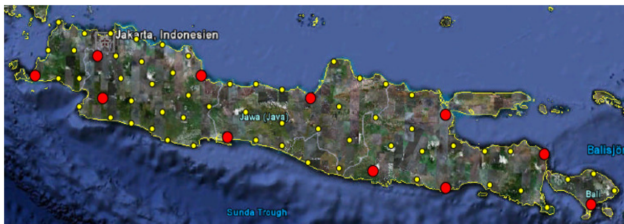
Figure 4. Planned location and distribution of BPN GPS CORS station in Java [Adiyanto and Wibisono, 2009]. Class-A and Class-B stations are denoted with red and yellow circles respectively.
