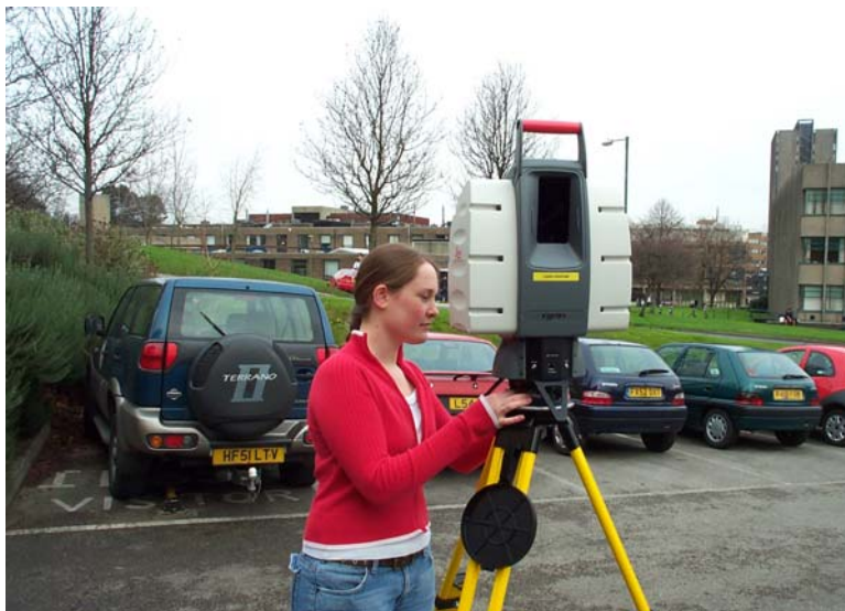
Figure 1: the Leica HDS3000 being set up at the University
