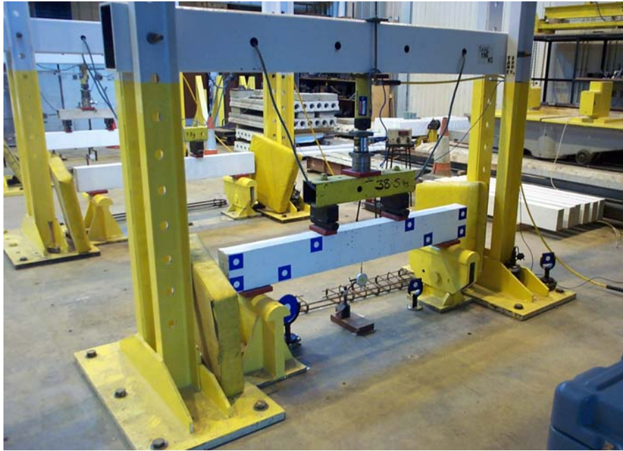
Figure 2: the concrete beam before loading with targets attached.
