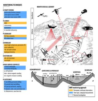
Figure 3. Multi-technique monitoring strategy at OMIV Landslide Observatory (<u>http://ano-omiv.cnrs.fr</u>).
