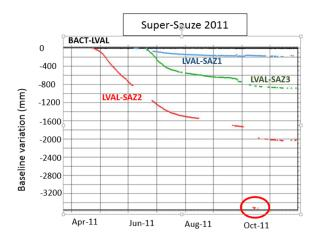
Figure 7. Example of anomalous estimation of baseline changes at Super-Sauze landslide (French Southern Alps) (Boetzlé, 2015).
