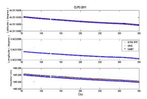
Figure 9. Comparison of time series obtained through SCRS-PPP, GINS and GAMIT/GLOBK softwares for a rapid landslide (Boetzlé, 2015).
