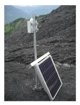
Figure 5. Geomon low-cost GNSS receiver and its solar panel on the Super-Sauze landslide (Boetzlé, 2015).
