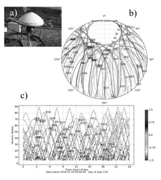
**Figure 4:** a) Antenna installation in station LEPE, b) skyplot example and c) time-elevation plot example of multipath, for station LEPE
