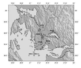
**Figure 3:** Station location of the GNSS Network PPGNet in Aitolo-Akarnania, in relation to active fault systems in the area. The simplified fault traces have been taken from Pérouse et al., 2017.
