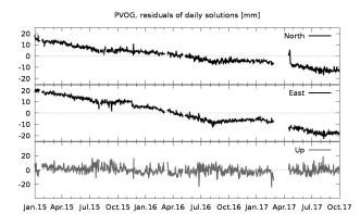
**Figure 5:** Example of coordinate time series for station PVOG. Residuals from average coordinates are displayed: Top panel, north component, middle panel east component, bottom panel up component. A slope and periodicities are clearly visible in north and east components.
