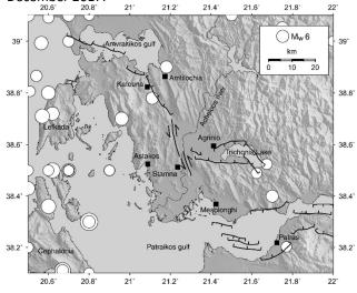
**Figure 2:** Tectonic map of Aitolo-Akarnania. The Katouna – Stamna sinistral fault and the Trichonis lake normal faults are shown. Seismicity is taken from Papazachos et al, 2010, (time period 1900-2010, events with M>5.5 are presented). Major cities are also shown. The simplified fault traces have been taken from Pérouse et al., 2017.
