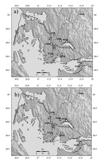
**Figure 6:** First results of the PPGNet, a) arrows denote relative movement of stations with respect to fixed PATR/PATO stations, b) relative movements with respect to fixed PVOG station, black lines indicate the main active faults in the area. The simplified fault traces have been taken from Pérouse et al., 2017.
