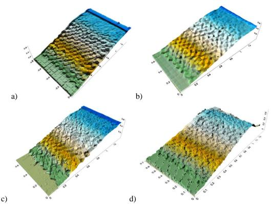
Fig. 3 Model envelope obtained with the four different methodologies. a) Kinect sensor b) MicMac software c) Python Photogrammetry Toolbox and d) Stereo photogrammetric reconstruction of submerged scenes
