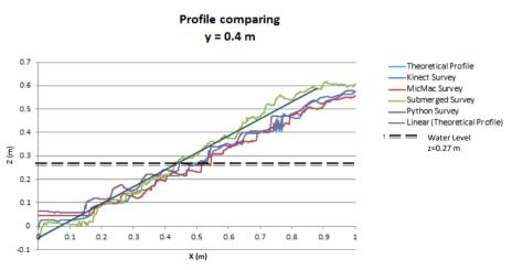
Fig. 4 Profile comparing using the four methodologies
