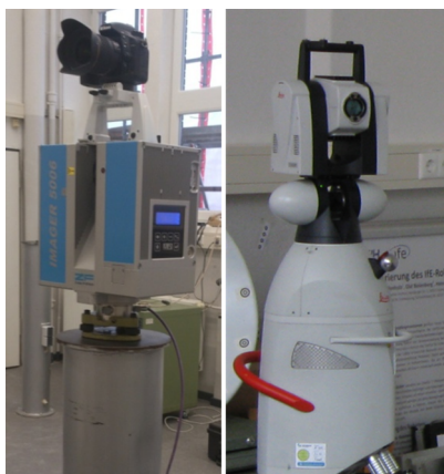
Fig. 1 A Nikon D750 24.3-megapixel digital camera is rigidly mounted on top of the Z+F Imager 5006 TLS (left), Leica AT901LR LT (right)
