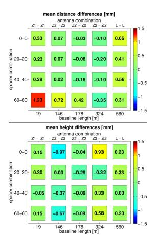
Fig. 2 Distance differences (top) and height differences (bottom) for dataset *equal*.
