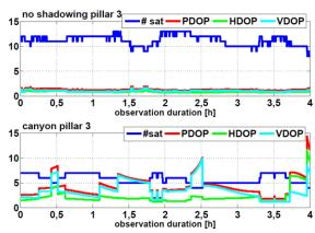
**Fig.** 7 Number of visible satellites (blue) and DOP values (PDOP red, HDOP green, VDOP cyan) for the non-shadowed case (top) and scenario *canyon* (bottom).
