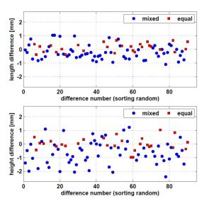
**Fig. 3** Comparison of distance differences (top) and height differences (bottom) for datasets *equal* (red squares) and *mixed* (blue circles).
