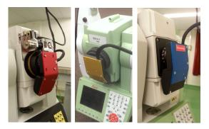
Fig. 1 CCD camera plugged on a TDA5005 (left), TS15 (middle), MS50 (right).
