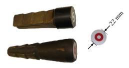
Fig. 4 Standard swisstopo target for dams.
