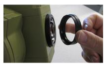
Fig. 2 Divergent lens plugged on the objective.
