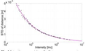
Fig. 1 Intensity vs. precision of a distance measurement
