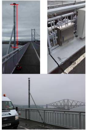
Fig.5 GeoSHM antenna setting-ups at middle span sites
