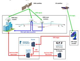
Fig. 2 The GeoSHM System Design
