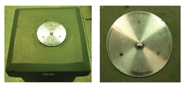
Figure 3 The head of pillar with centring plate
