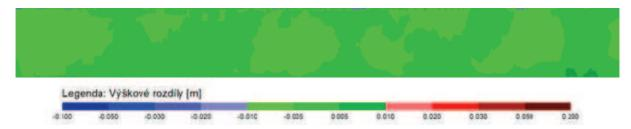
Figure 10 From the sample of differential DTM AFTER LAYING OF ASPHALT LAYER, it is obvious that it managed to perform the laying of the asphalt layer in tolerance with 3D projectfrom 99.6%
