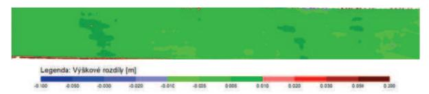
Figure 8 From the sample of the differential DTM it's seen that it managed the roadmilling in tolerance with 3D design from 98.4%
