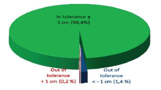
Figure 9 State after milling
