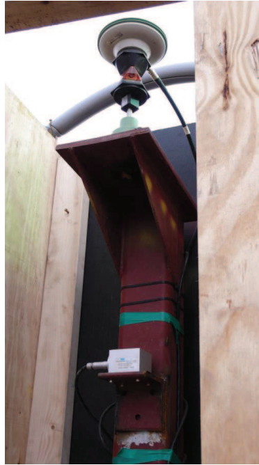
Figure 4 Collocated Active Prism and inclinometer (Whitworth, 2010)
