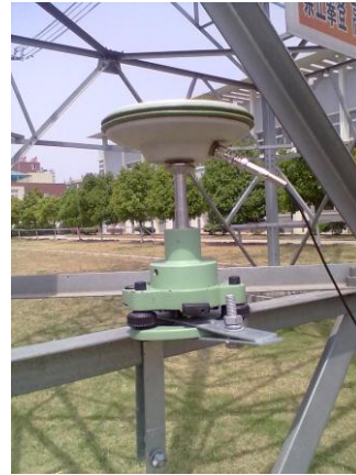
Figure 2. Photo of fixed antenna
