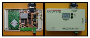
Figure 1 - GPS CAM-SYNC box – inside and cover
