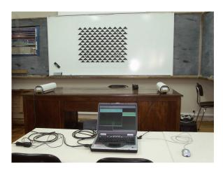
Figure 4 - Image acquisition to obtain calibration parameters of the video camera lenses.
