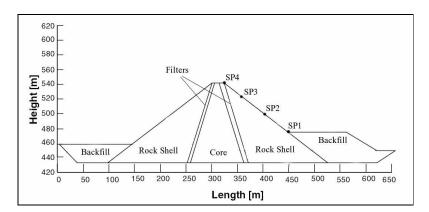
Figure 3 - West Dam cross section
