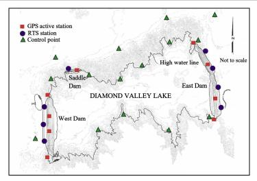
Figure 1 - Geodetic monitoring scheme at the DVL project
