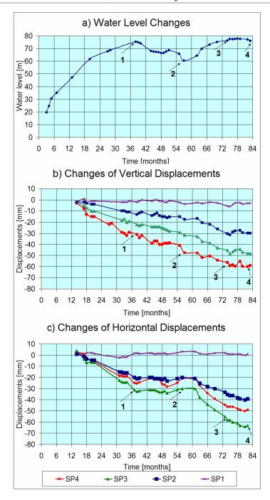
Figure 5 - Water level and displacement changes as a function of time
