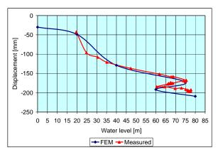
Figure 6 - Modeled and measured settlement of pt. SP4 as a function of water level
