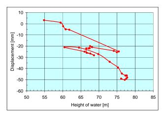
Figure 7 - Measured changes of horizontal displacements of pt. SP4
