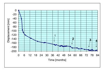
Figure 4 - Measured settlement of point SP4 as a function of time
