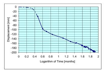
Figure 5 - Measured settlement of point SP4 as a function of log (time)
