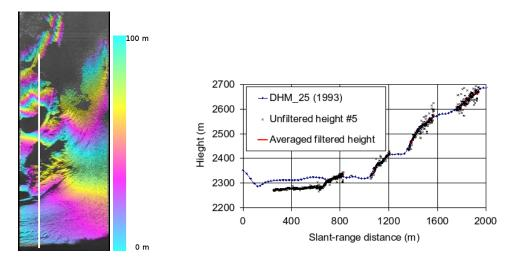
Figure 6 left - Height map in radar geometry (azimuth versus slant range = distance from sensor). The white line indicates the selected transect. Right - Height profiles of the radar height map of 2007 and the Swisstopo DHM25 heights of 1993 along the transect.
