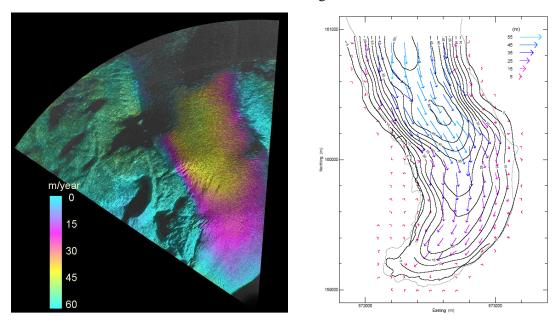
Figure 5 Left - Displacement map estimated from 4 interferometric pairs with a total time span of 80 minutes in map projection. Right - Yearly flow direction and speed derived from photogrammetry (Bauder, personal communication).
