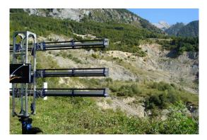
Figure 1 left - GAMMA terrestrial radar interferometer. Right - Target area.
