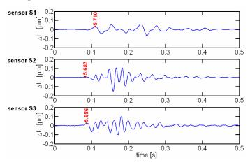
Figure 6 - Relative movements of the concrete anchors caused by a hammer impact
