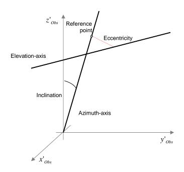
Figure 1 - Restrictions (eccentricity and inclination), for clearness shown in the coordinate system  $x'_{Obs}$ ,  $y'_{Obs}$ ,  $z'_{Obs}$ , which emantes from the observation system  $x_{Obs}$ ,  $y_{Obs}$ ,  $z_{Obs}$  by translation
