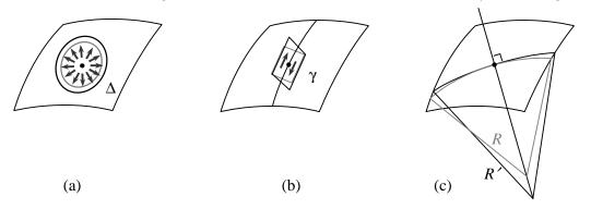
**Figure 1**: Three modes of surface deformation: (a) dilatation (area variation), (b) maximum shear and (c) bending expressed by the change of the radii of curvature of normal sections
