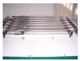
Figure 3 - Interior wire extensometer.
