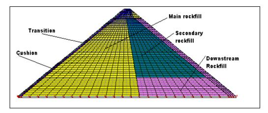
Figure 2 - Shibuya Dam, FEM mesh and dam zoning.
