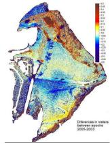
Figure 8 - Settlements - 2005 epoch as compared to 2003.
