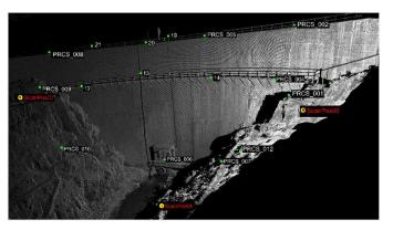
Figure 1 - A perspective of the laser intensity 3D model of Alto Ceira dam downstream face, layout of stations (with red labels) and retro-reflector targets (with white labels).
