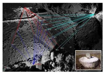
Figure 6 – Laser intensity 3D point cloud of the Lapão Dam (2007) showing the 3 scan positions, retro-reflector targets and vectors between scan positions and surface marks. The smaller image is a retro reflector target on forced centering materializing an object point
