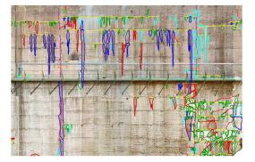
Figure 2 - Ortoimages as a base map for heads up vectorisation of anomalies classified and symbolised according to a catalogue.
