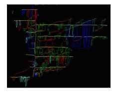
Figure 3 - Vectorisation of cracks, spalling, leaching, leakage, indicators of chemical reactions, erosion or cavitation according to a predefined legend.
