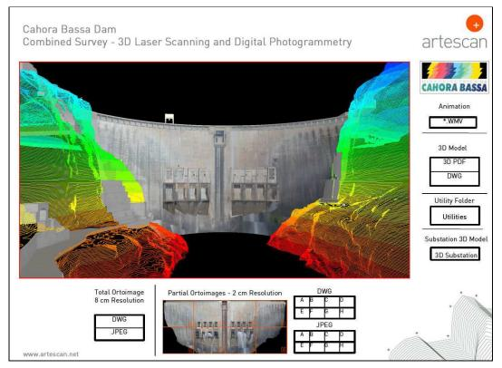
Fig. 10 – PDF Application with embedded 3D CAD model of Cahora Bassa dam and its near slopes.
