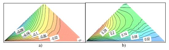
Figure 2 - Predicted displacements [m] after filling the reservoir a) vertical displacements b) horizontal displacements
