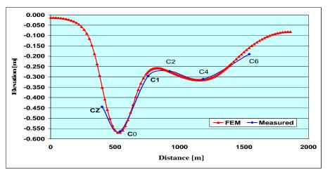
Fig.6: Measured and FEM Surface Subsidence
