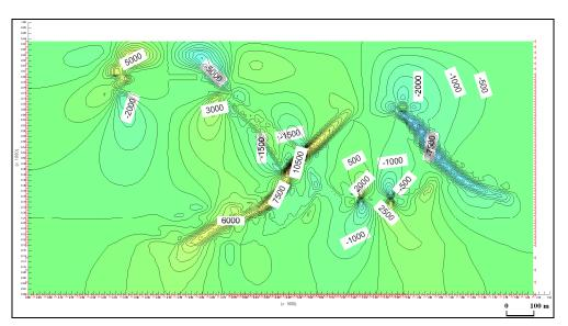
Fig. 7 - Distribution of maximum shearing stress (MPa)
