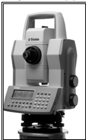
Photo1: The total station Trimble 5605 DR +
