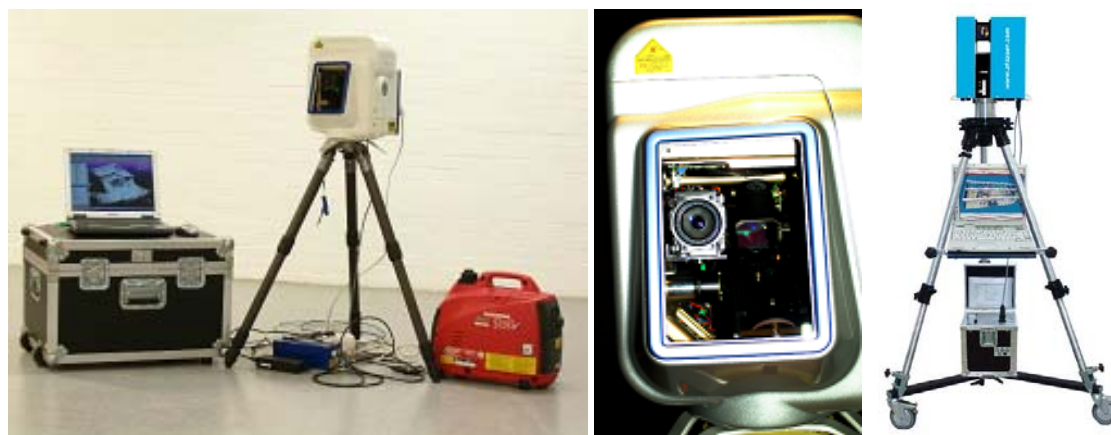
Fig. 1: 3D laser scanning system Mensi GS100 of the HCU with accessories (left), GS100 interior with digital camera and mirror (middle), IMAGER 5003 with accessories (right)
