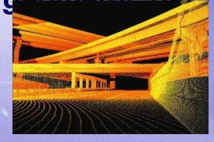
Utilizing 3D laser technology, HDS captures, visualizes and models complex structures and sites with an unprecedented combination of completeness, speed, accuracy, and safety.
