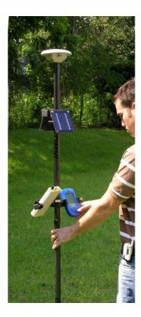
Figure 3. DataGrid Mk-1 Crane or Toughman GPS/Data colloctors in typical field configuration. Shown on a pole with low weight antenna, solar panels and a PDA.
