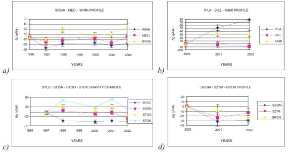
Fig. 3 Gravity changes of selected GEOSUD profiles, located near the dams: a)Słup Dam, b) Bielawa Dam, c) Kamieniec Dam (designed), d) Dobromierz Dam
