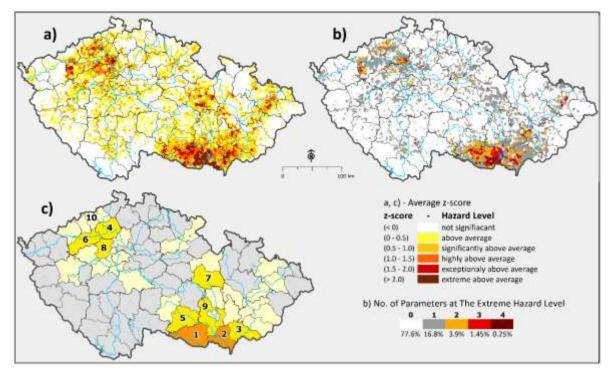
Figure 9. The result of the multiple-hazard analysis at the cadastre (a-b) and district (c) level: a) mean z-score of all six individual hazards, b) number of individual hazards per cadastre unit in the worst category, and c) the districts with the highest combined hazard level within the country. The top 10 regions according to hazard level are numbered.
