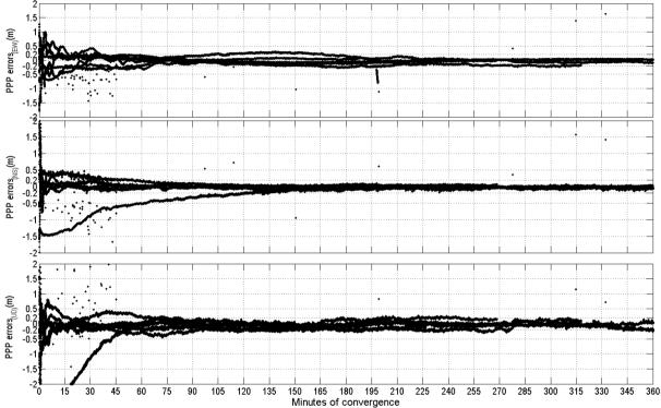
**Figure 8.** Performance of kinematic PPP using MADOCA-LEX products. RMS positioning errors after 2 hours of convergence E/N/U: 0.081cm/0.036cm/0.115cm
