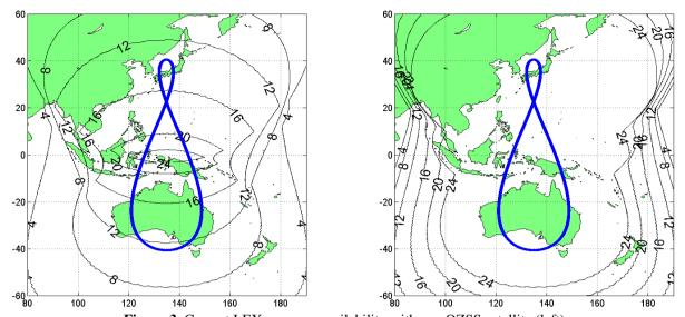
**Figure 3.** Current LEX message availability with one QZSS satellite (left). Expected LEX message availability with 3 active HEO satellites in 2018 (right).
