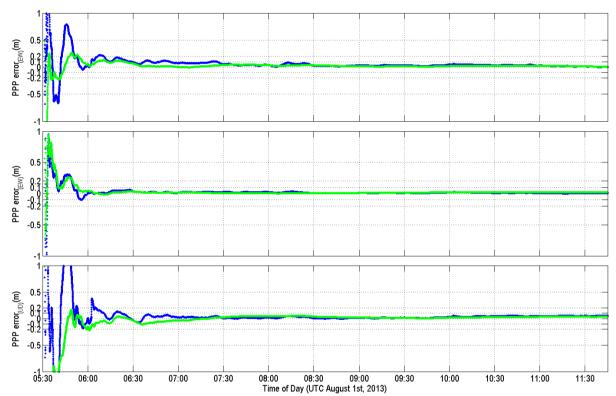
**Figure 7.** Performance of static PPP using MADOCA-LEX products (Blue) and IGS-RT products CLK11 (Green). RMS errors were E/N/U: 0.029m/0.012m/ 0.026m for MADOCA-LEX. E/N/U: 0.019cm/0.017cm/0.024cm for IGS-RT.
