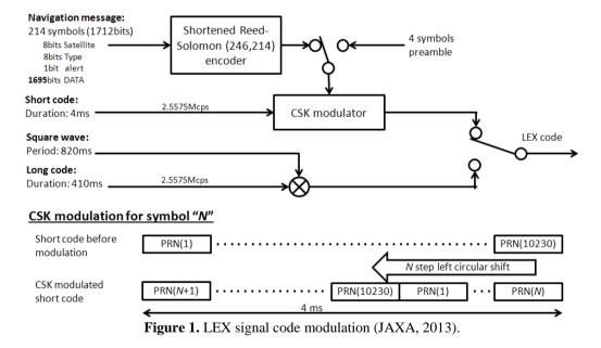
The LEX signal uses a Kasami series short code (2.5575 Mcps) with a chip length of 10230 and a 4 ms period, and a Kasami series long code (2.5575 Mcps) with a chip length of 1048575 and a 410 ms period. The short code is modulated by the navigation message using a 256-ary Code Shift Keying (CSK), which consists in replacing the short code with a left circle shifted version of it, the number of steps to be shifted representing the symbol value (JAXA, 2013).
