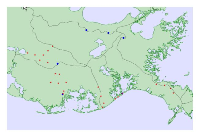
**Fig 4.1** The sessions of a project are listed in a dialog box along with the rover and reference stations for each session. A dynamic map is also generated which illustrates the rover and reference stations as each session is selected.
